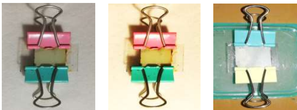
Figure 11 DSSCs with alligator clips
