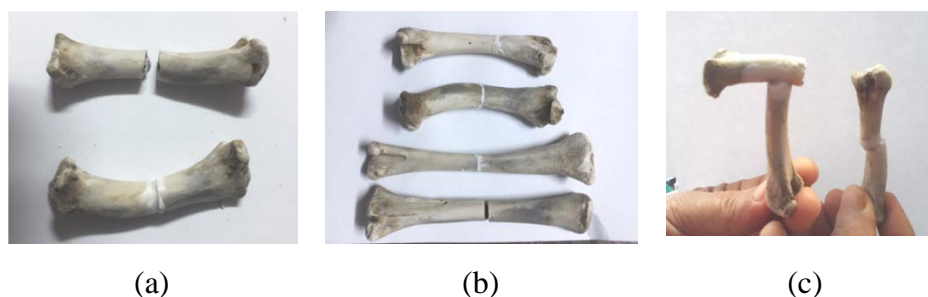
Figure 3.14 HAp-10 % MgO nanocomposite (1100 °C) as bone glue for broken chicken femur bone
