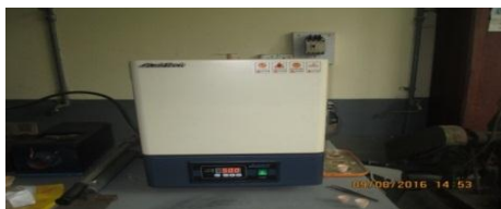
(A). Ashing samples in furnace
