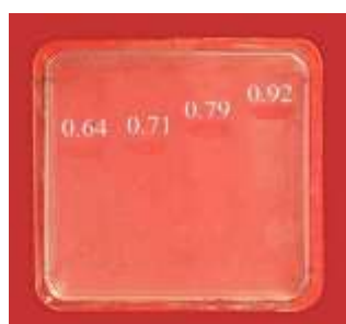
Figure 12 Paper chromatography bioautographic assay
