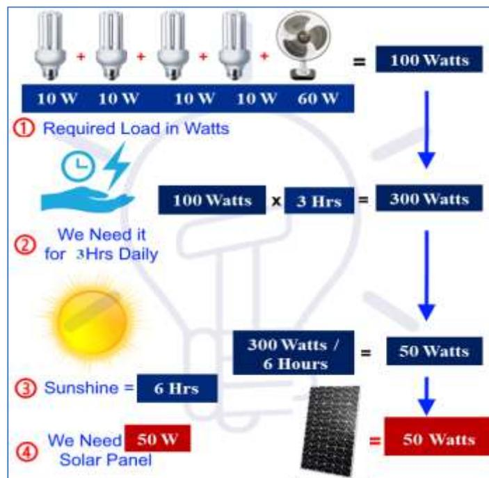
**Figure 13** The block diagram of the uses of home appliances for 50 W solar panel
