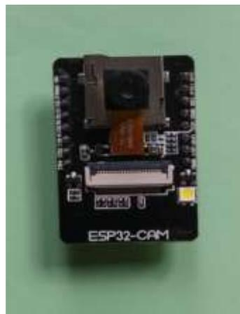
**Figure 3** The photo of ESP32\_CAM
