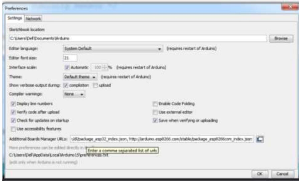
Figure 5 Including ESP8266 board
