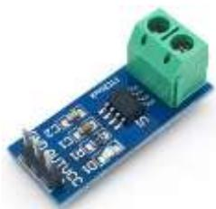
**Figure 5** Component of current sensor module
