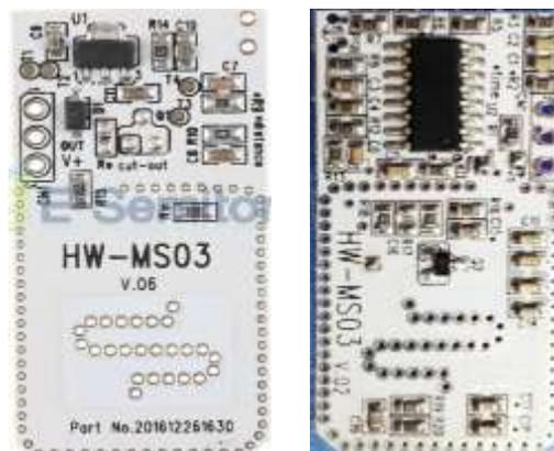
**Figure 2** Microwave sensor HW MS03
