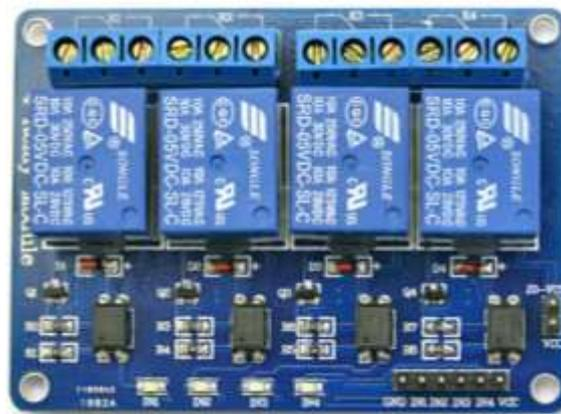
**Figure 3** 4-channel relay
