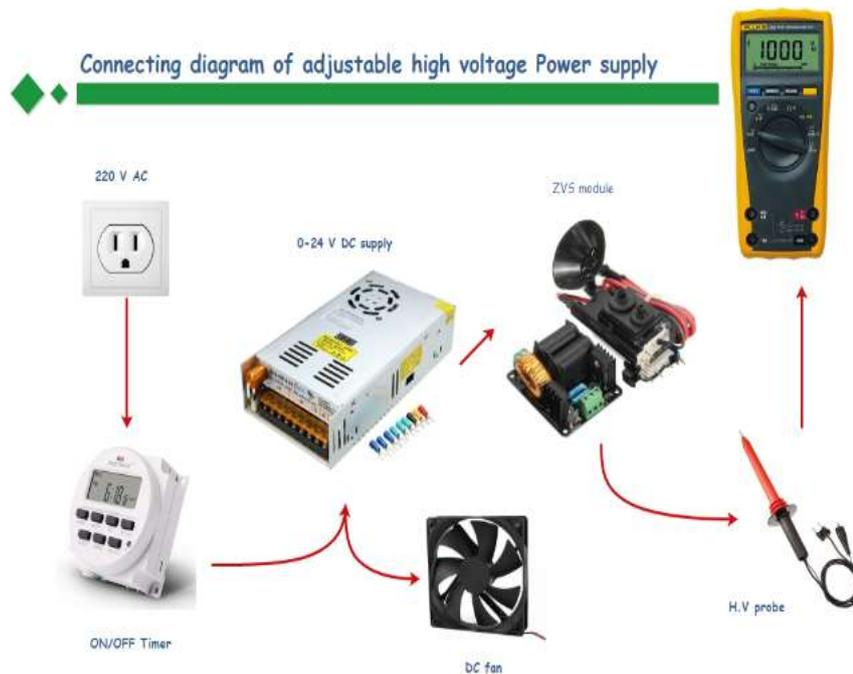
**Figure 1 (a)** The connecting diagram of automatic on/off variable HV power supply
