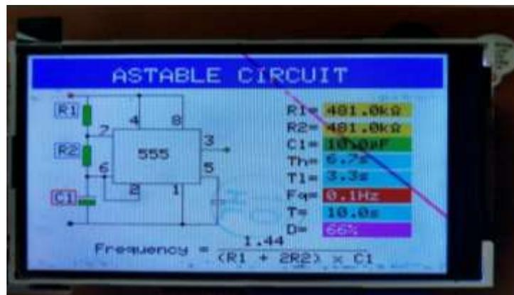
Figure 12 The calculated results for astable circuit
