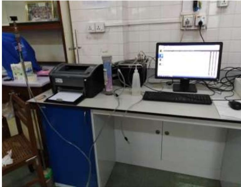
**Figure 5** The photograph that was measuring soil sample with RAD 7 detector connected to PC.
