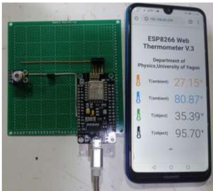
**Figure 7** Contactless thermometer
