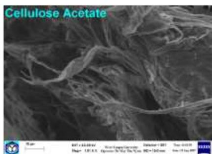
**Figure 3** SEM photomicrograph of cellulose acetate
