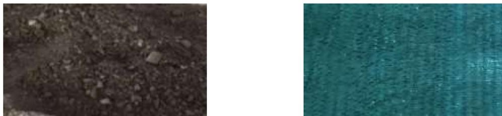
**Figure 5** Charcoal used in slow sand filtration system **Figure 6** Mesh to prevent mixing of the gravels and the coarse sand
