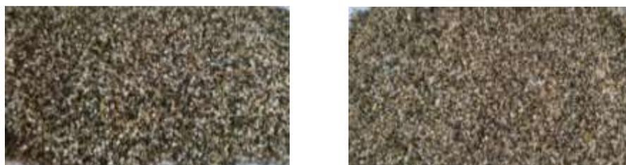
**Figure 3** Different size gravel (average 5 mm and 2 mm in diameter) used in slow sand filtration system
