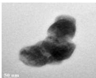
**Figure 6** TEM image of Fe<sub>3</sub>O<sub>4</sub>-ZnO-CuO nanocomposites
