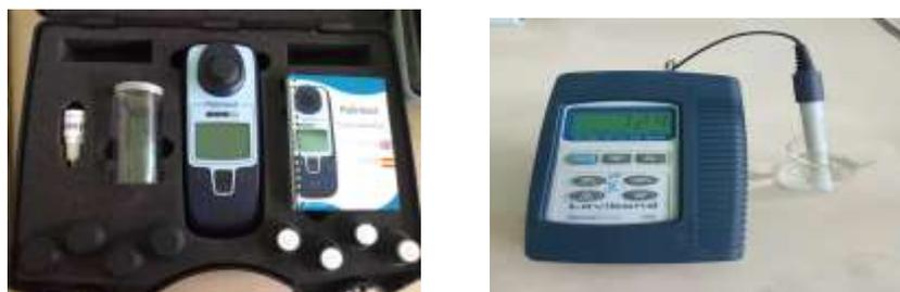
**Figure 5** Turbidity apparatus and pH meter
