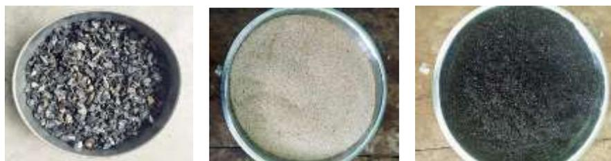
**Figure 2** Chipping stones, rice husk char and sand for water treatment
