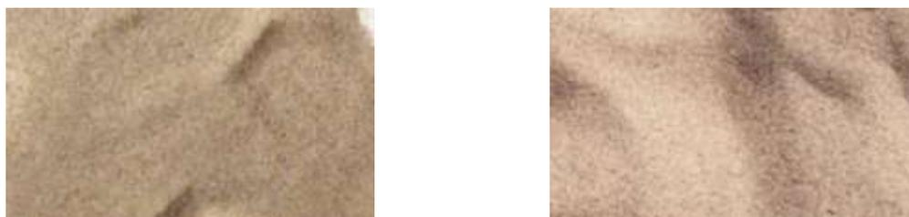
**Figure 4** Fine sand and coarse sand used in slow sand filtration system
