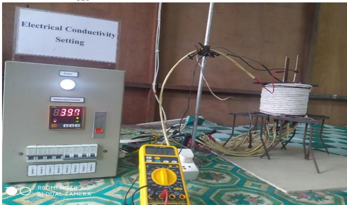
**Figure-4** Temperature dependent electrical resistances measurement
