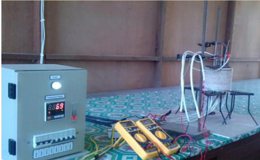
**Figure.4.** Temperature dependent electrical conductivity measurement
