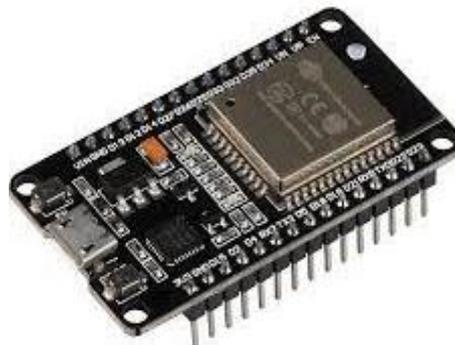
**Figure 2.** Photograph of ESP-WROOM 32 microcontroller board
