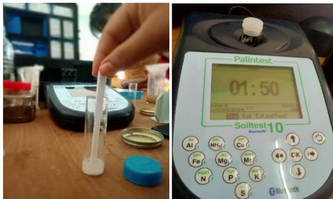
Figure 12 Procedure of K (Potassium Test)
