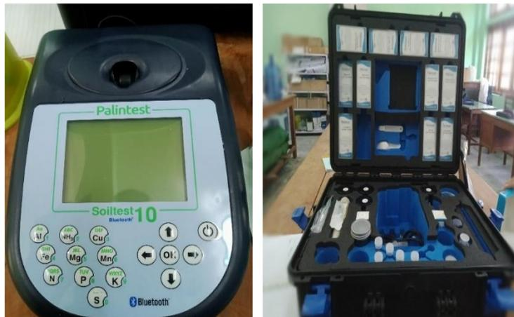
**Figure 9** Photographs of Soiltest 10 photometer and Chemical box
