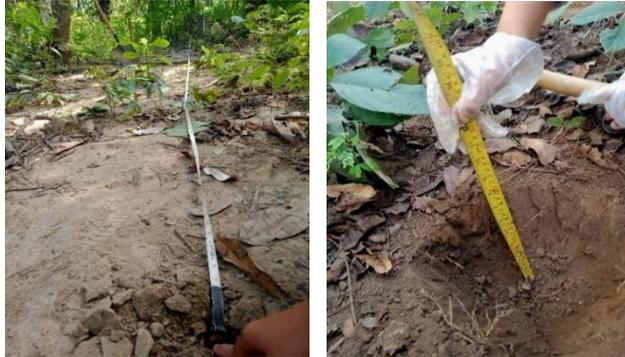
Figure 1 Photographs of soil samples with the depth of 6 inches
