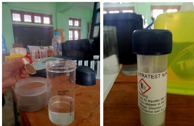
**Figure 10** Procedure of N (Nitrogen Test)
