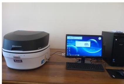
**Figure 1** Energy Dispersive X-rays Fluorescence (EDXRF) spectrometer (EDX-7000)
