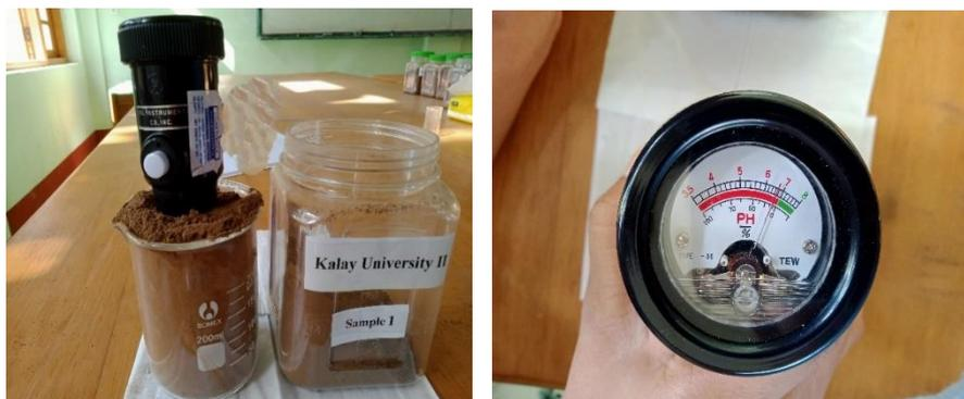
**Figure 6** Photographs of measured the pH (potential hydrogen) of soil sample.
