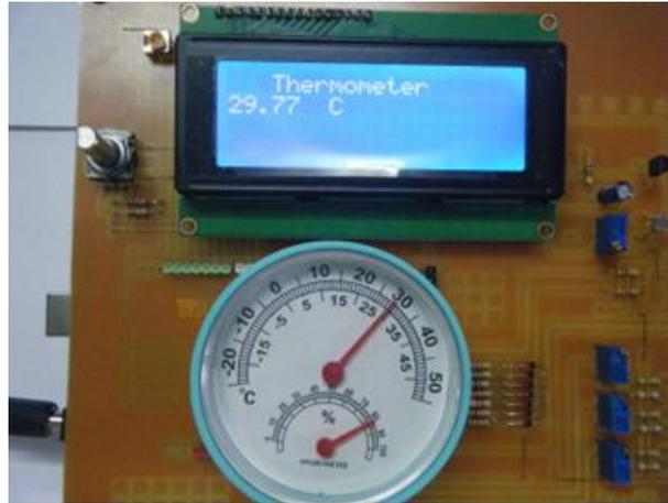
**Figure 10:** Photograph of measuring results for temperature
