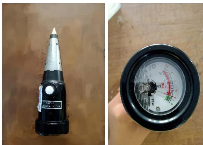
**Figure 5** Photographs of Kelway Soil Acidity and Moisture Tester
