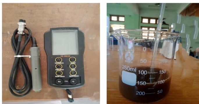
**Figure 7** Photograph of HI 8633 Conductivity Meter
