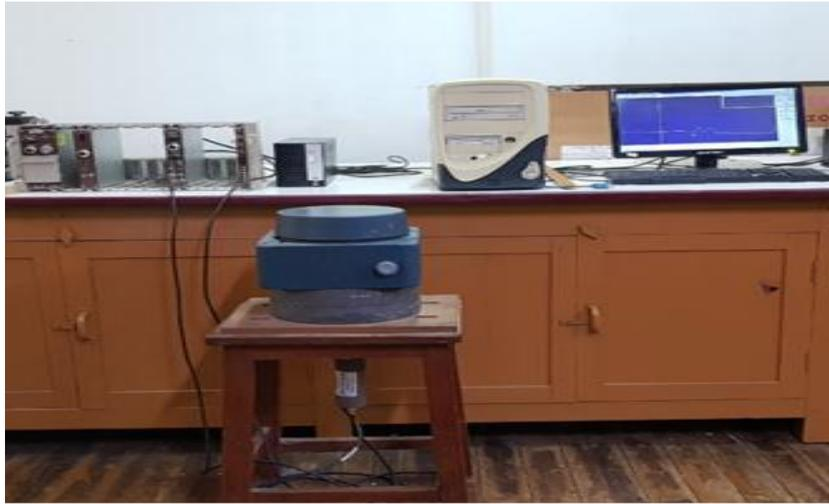
**Figure 4.** Experimental Set-up for Gamma Radiation Measurement
