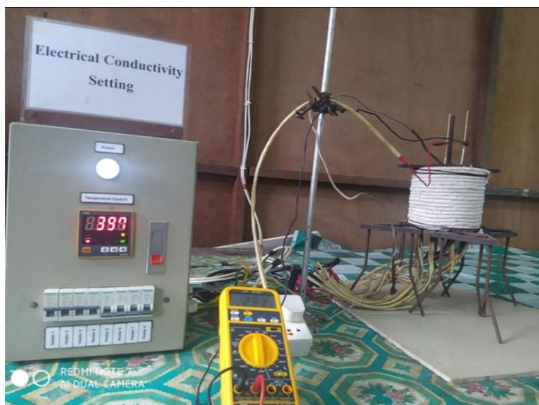
**Figure 6** Experimental set-up of resistivity measurement
