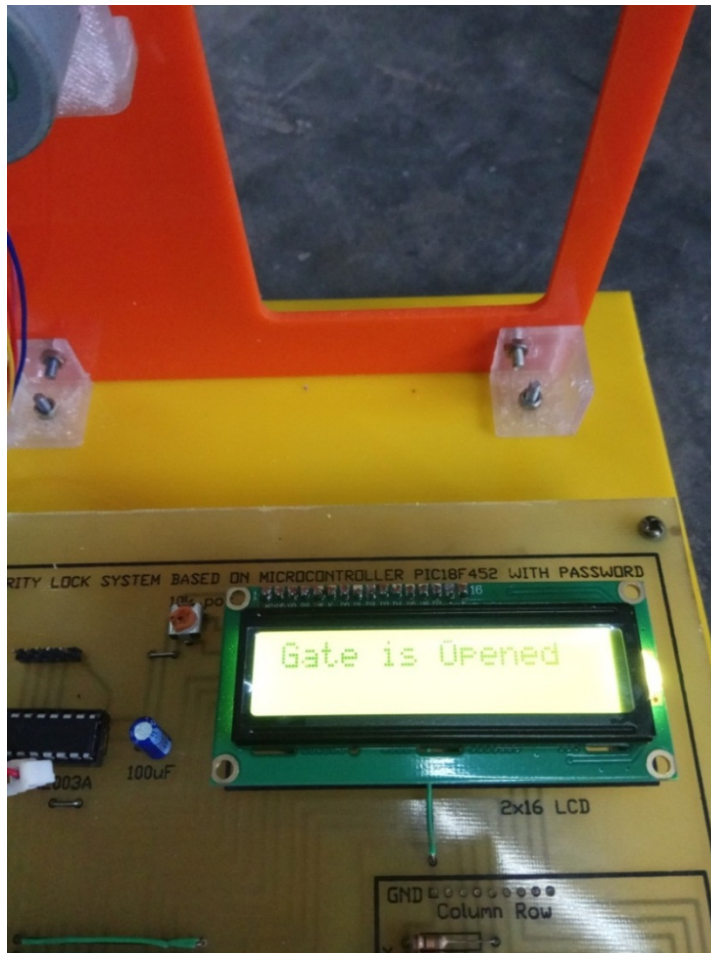
Figure 17 Gate open stage of security lock system
