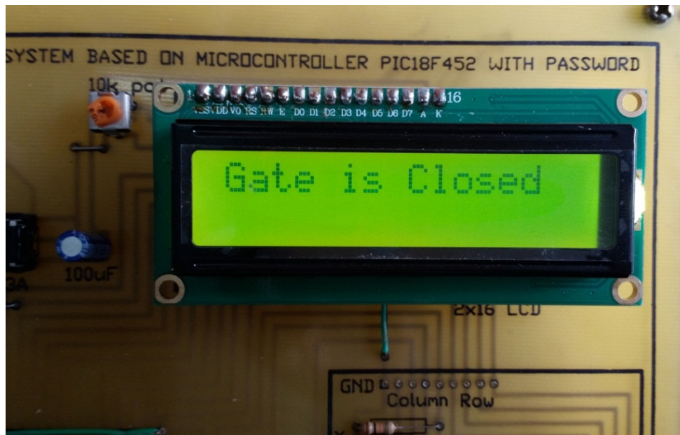
Figure 18 Gate close stage of security lock system
