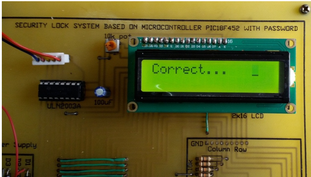
Figure 16 Entering correct password stage
