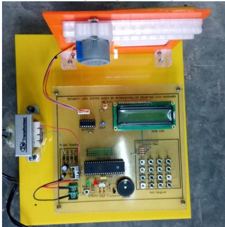
Figure 14 Photo of security lock system
