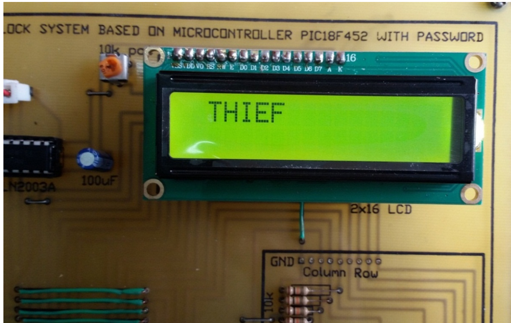
Figure 20 Entering incorrect password three times
