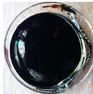
Figure 3 Photo of P(Py-2FPy)/ZnO composite film casted in the Petri dish
