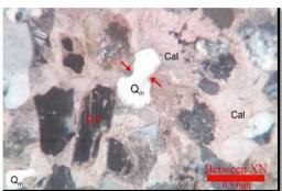
**Figure 13.** Photomicrograph showing calcite cement (Cal) corroded by monocrystalline framework grain dissolution has been quartz (Q<sub>m</sub>) of sandstone in Shwezetaw Formation
