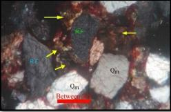
**Figure 10.** Photomicrograph showing chlorite rims around the detrital grains (arrow) of sandstone in Shwezetaw Formation
