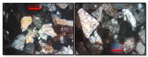
**Figure 17.** Photomicrograph shows point contacts, porosity and permeability nature (arrow) of sandstone in Shwezetaw formation
