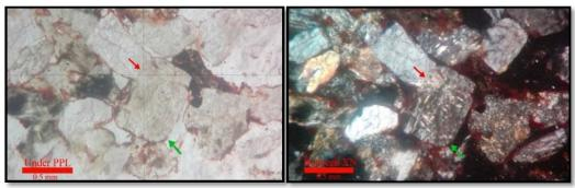
**Figure 12.** Photomicrograph showing absence of hematite coating at grain contacts(red arrow) and late hematite coating is on detrital grains boundary (green arrow) of sandstone in Shwezetaw Formation
