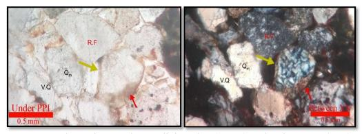
**Figure 11.** Photomicrograph pore lining clay (arrow), volcanic quartz (V.Q), monocrystalline quartz (Q<sub>m</sub>) of sandstone in Shwezetaw Formation
