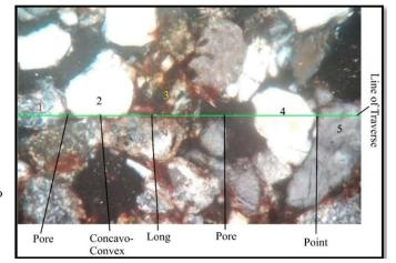
Packing Proximity =  $\frac{\text{Total number of contacts encountered } 3 \times 100}{\text{Total number of grains encountered 5}}$
