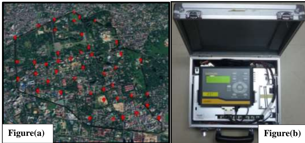
Figure 4 Geophysical Measurement of the research area, (a).Locations of microtremor measurements in Dagon Township, Yangon, (b) SMAR-6A3P Microtremor Equipment and Microtremor Surveying
