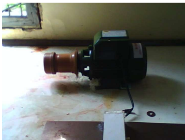
Figure 2.(e) Photograph of the laboratory-made ball-milling machine
