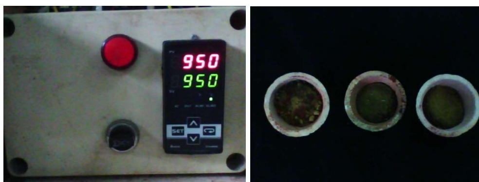
Figure 2. Photographs of the (j) DELTA A Series Temperature Controller DTA4896 at 950°C and (k) as-prepared BaFe 2 O 4 prepared at 950°C
