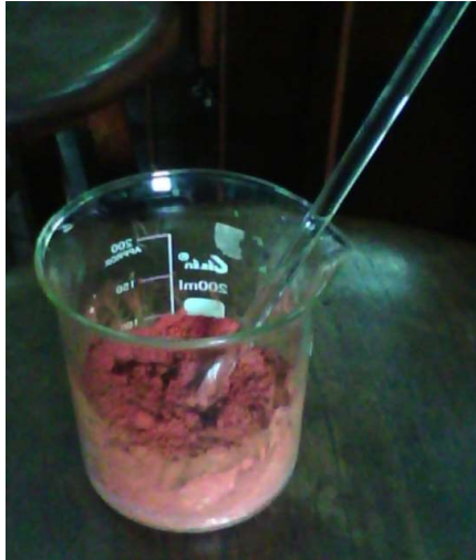
Figure2.(b) Photograph of the mixed weighed starting materials of \text{Fe}_2\text{O}_3 and \text{BaCO}_3
