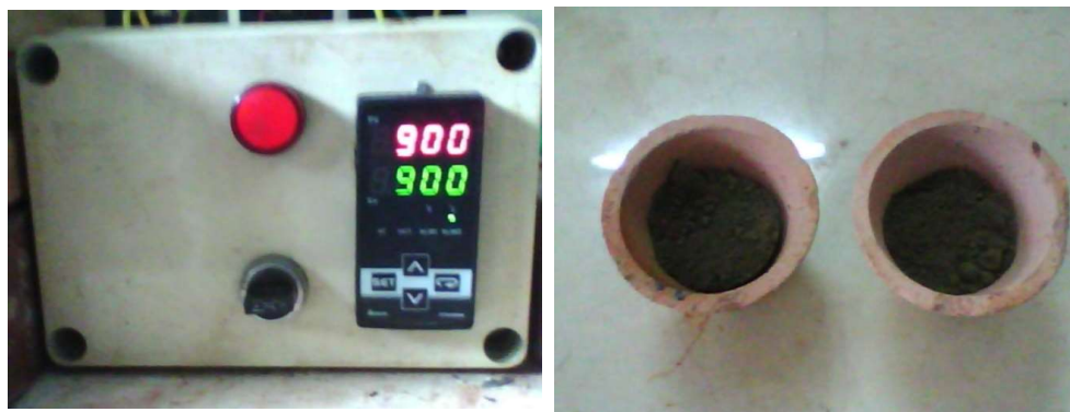
Figure2. Photographs of the (h) DELTA A Series Temperature Controller DTA4896 at 900°C and (i) as-prepared BaFe 2 O 4 prepared at 900°C
