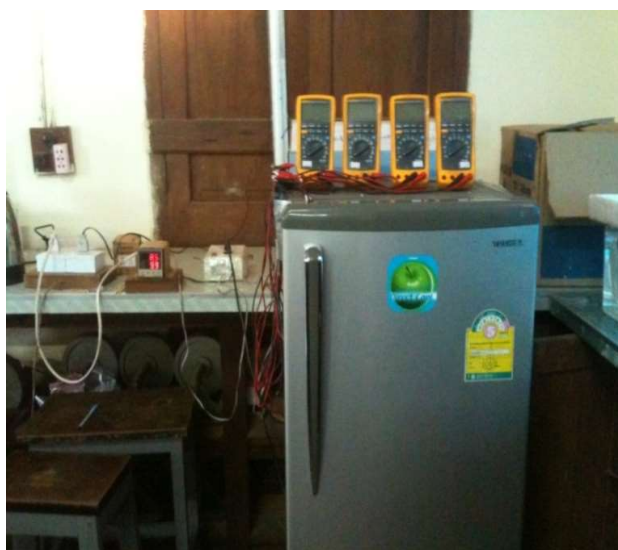
Figure 3.(b) Photograph of the experimental setup of humidity sensitive electrical properties measurement
