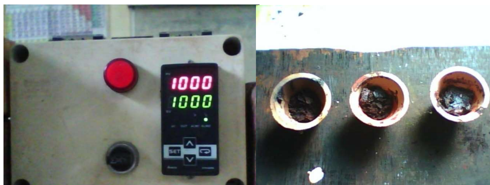
Figure 2. Photographs of the (l) DELTA A Series Temperature Controller DTA4896 at 1000°C and (m) as-prepared BaFe 2 O 4 prepared at 1000°C
