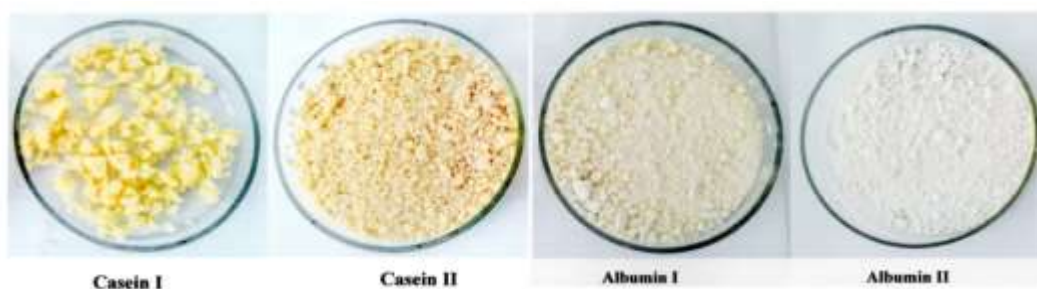
Figure 2 Isolation of casein I, II, albumin I and II from fresh and packed cow milk samples
