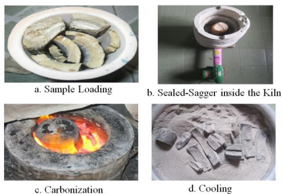
Figure 4 Processing of White Charcoal by Forced Air Type Updraft Kiln with Sagger
