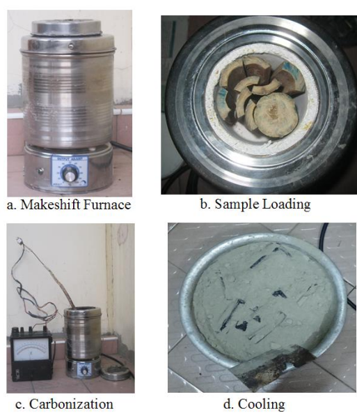
Figure 6 Processing of White Charcoal by Makeshift Furnace
