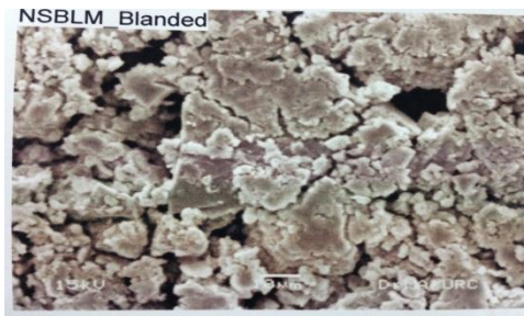
Figure 13: SEM micrograph of the blended cement (BC) sample at 1000 × magnification
