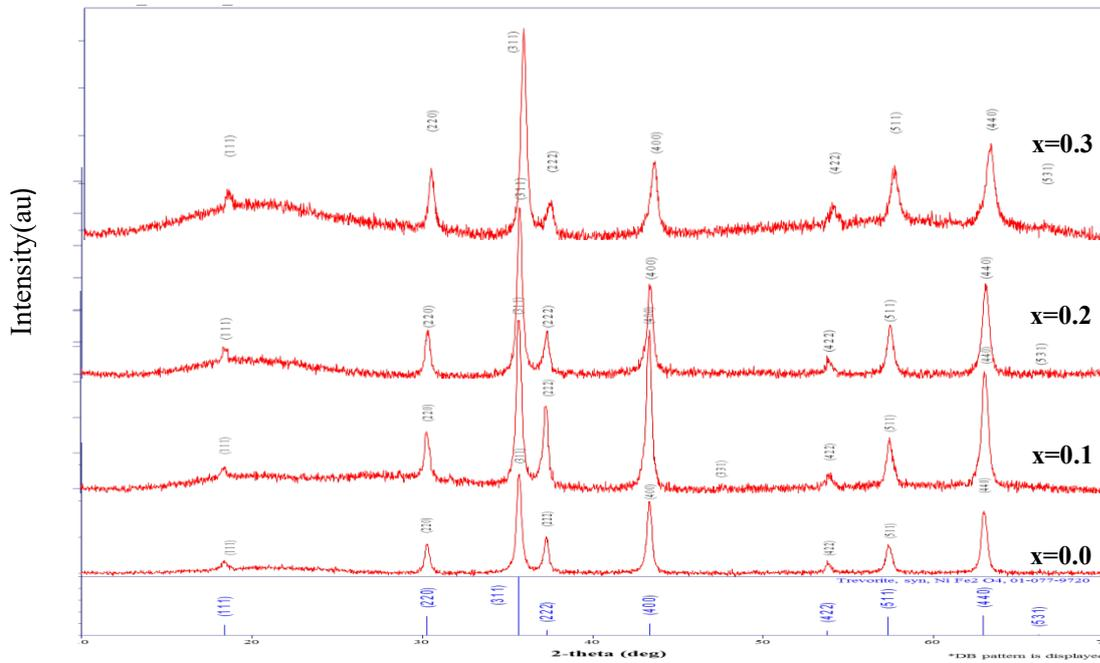
**Figure 3** (a) XRD Spectrum of Ni<sub>1-x</sub>Co<sub>x</sub>Fe<sub>2</sub>O<sub>4</sub>ferrites with different Co concentration by self-combustion method
