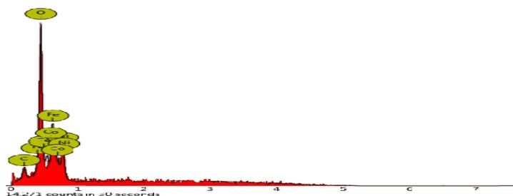
**Figure 5 (b)(iii)** EDS pattern of  $Ni_{1-x}Co_xFe_2O_4$  nanoferrite with different Co  $x = 0.2$  concentration by sol-gel method
