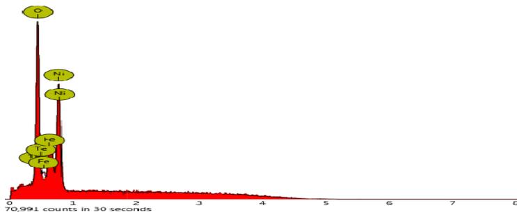
**Figure 5(a)(iii)** EDS pattern of  $Ni_{1-x}Co_xFe_2O_4$  nanoferrite with different Co  $x = 0.2$  concentration by self-combustion method
