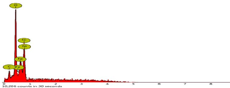
**Figure 5(a)(ii)** EDS pattern of  $Ni_{1-x}Co_xFe_2O_4$  nanoferrite with different Co  $x = 0.1$  concentration by self-combustion method
