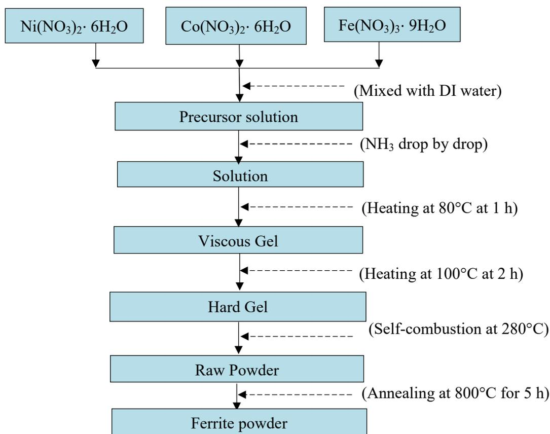
**Figure 1** Experimental sequence of Cobalt Doped Nickel ferrites for Self-combustion method
