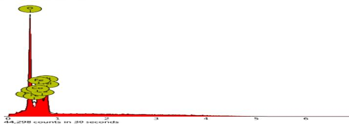
**Figure 5 (a)(iv)** EDS pattern of  $Ni_{1-x}Co_xFe_2O_4$  nanoferrite with different Co  $x = 0.3$  concentration by self-combustion method
