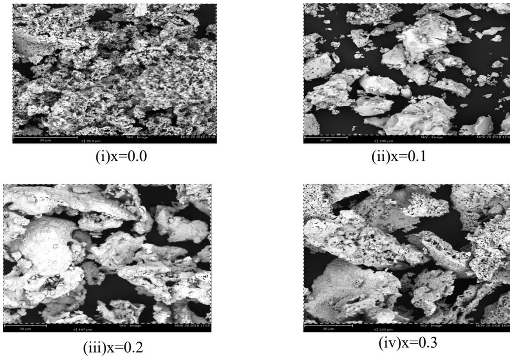
**Figure 4 (b)** Scanning electron images of  $Ni_{1-x}Co_xFe_2O_4$  nano ferrite with different Co concentration by sol-gel method
