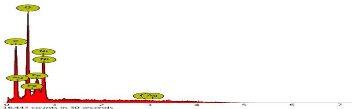
**Figure 5(b)(ii)** EDS pattern of  $Ni_{1-x}Co_xFe_2O_4$  nanoferrite with different Co  $x = 0.1$  concentration by sol-gel method
