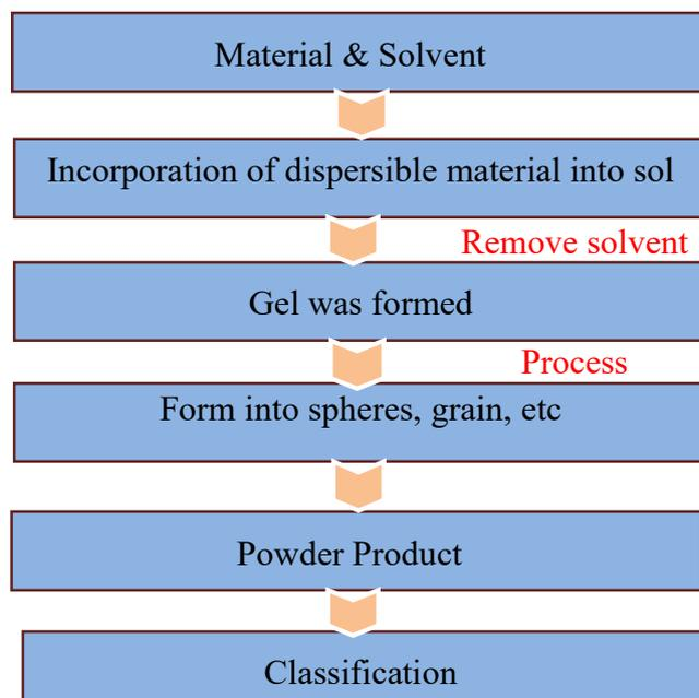
**Figure 2** The production steps for sol-gel production route
