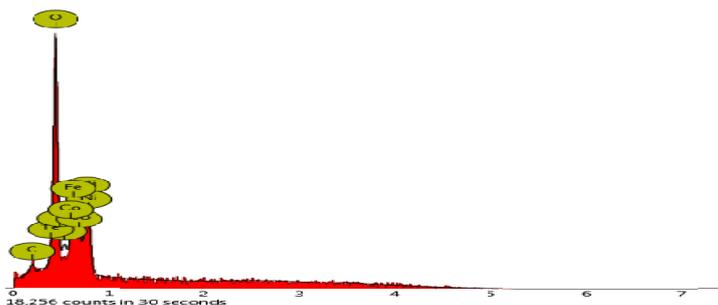
**Figure 5 (b)(iv)** EDS pattern of  $Ni_{1-x}Co_xFe_2O_4$  nanoferrite with different Co  $x = 0.3$  concentration by sol-gel method
