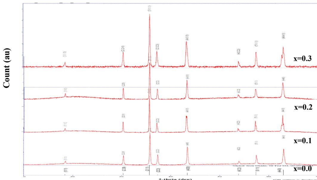
**Figure 3 (b)** XRD Spectrum of  $Ni_{1-x}Co_xFe_2O_4$  ferrites with different Co concentration by sol-gel method
