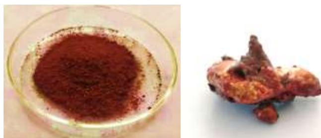
**Figure 8.** Extracted copper from the Letpadaung copper mine rock samples
