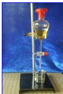
Figure 3 Extraction of antibacterial compound
