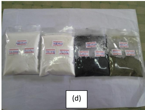
Figure 2:(d) Photograph of the weighed \text{Li}_2\text{CO}_3 , \text{CoO} and \text{NiO}
