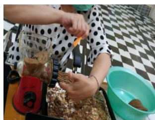
(G) Extruding of fish pellet
