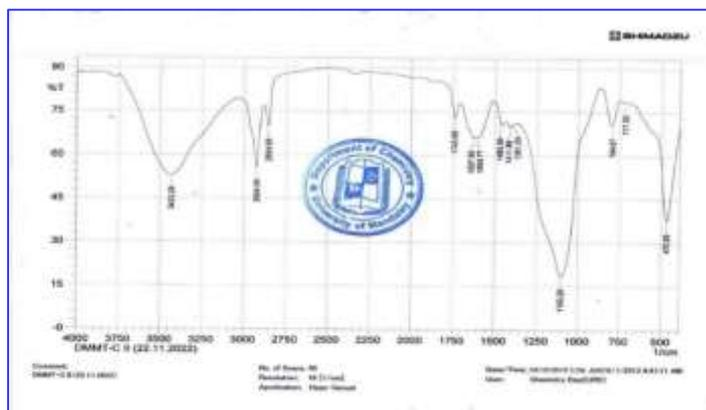
**Figure 10.** FT IR spectrum of metabolite-II
