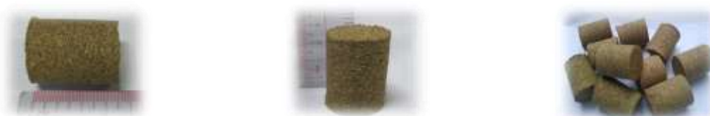
Figure 5 Appearance of fuel pellets densified by commercial scale
