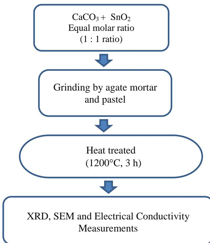
**Figure 1:** Flow diagram of the preparation of  $\text{CaSnO}_3$  sample
