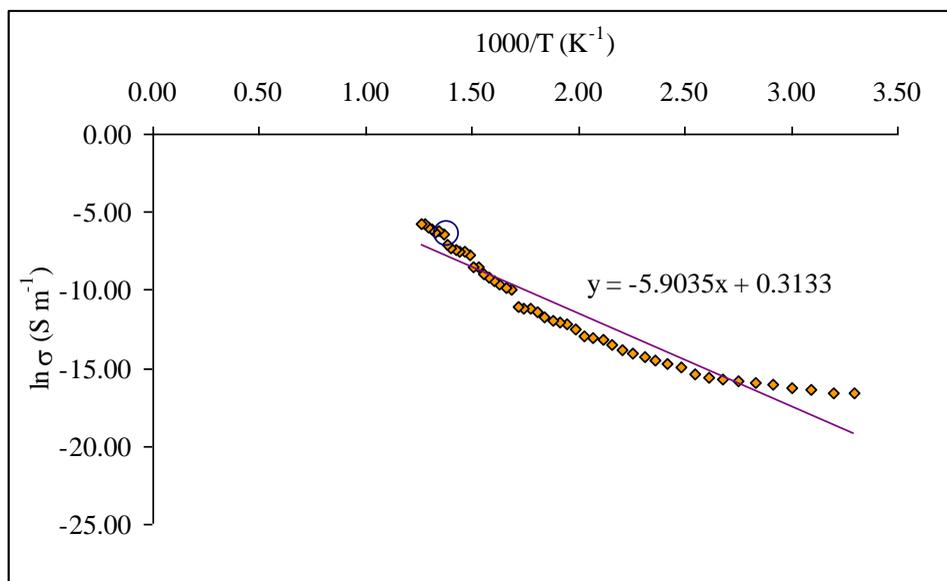
**Figure 10:** (c) Arrhenius plot of the dc electrical conductivity of the BaSnO<sub>3</sub>
