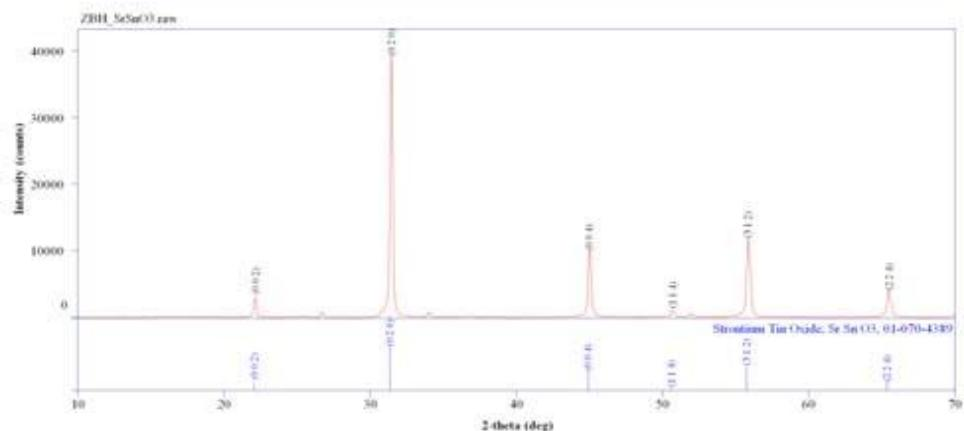
**Figure 5:** XRD pattern of SrSnO<sub>3</sub>
