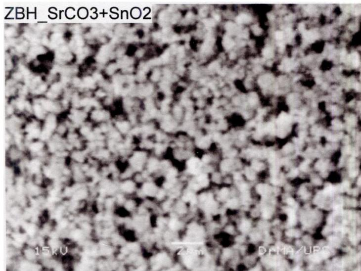
**Figure 8:** SEM micrograph of the SrSnO<sub>3</sub>
