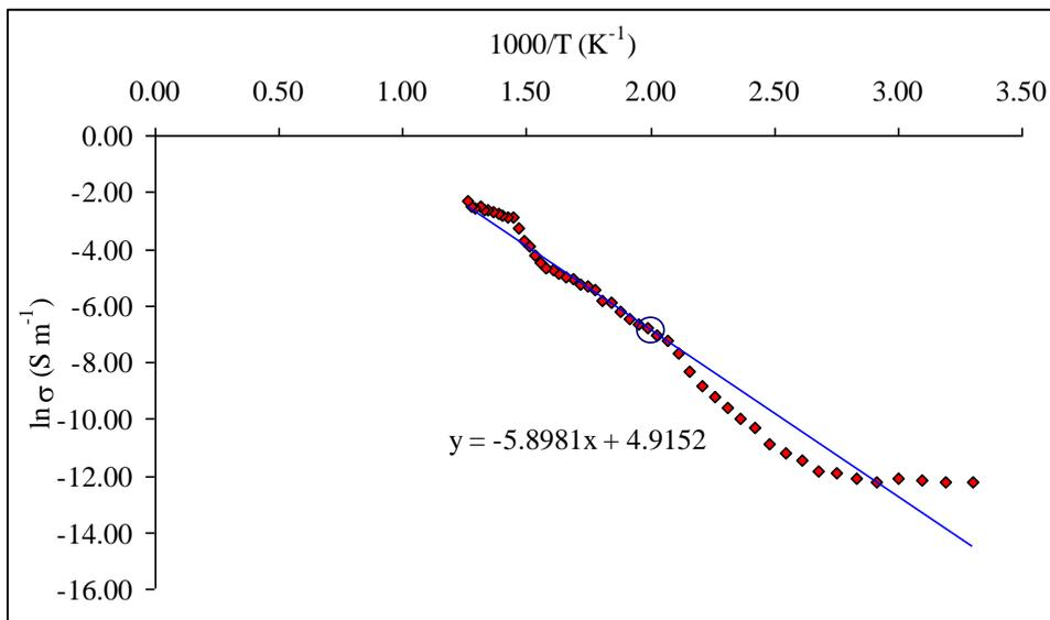
**Figure10:** (a) Arrhenius plot of the dc electrical conductivity of the  $\text{CaSnO}_3$
