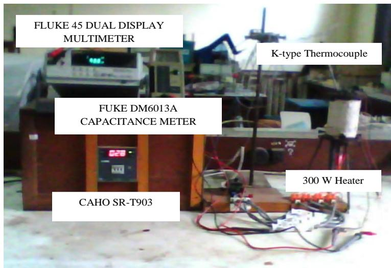
**Figure 2:** Photograph of the experimental setup for the temperature dependent electrical resistance measurement
