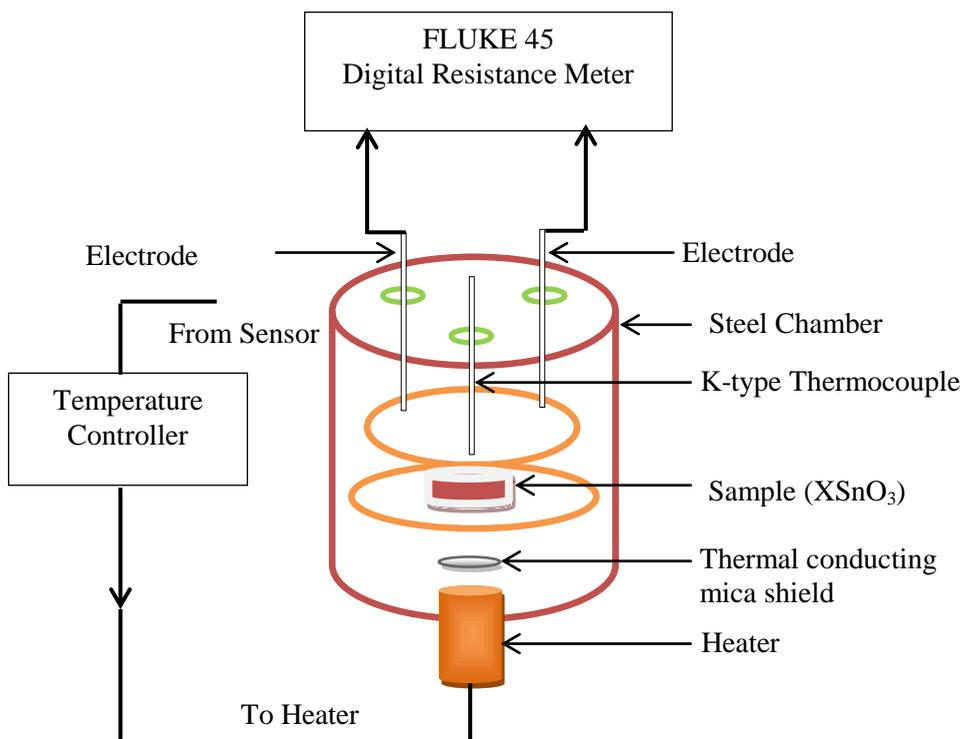
**Figure 3:** Schematic diagram of the experimental setup for the temperature dependent electrical resistance measurement
