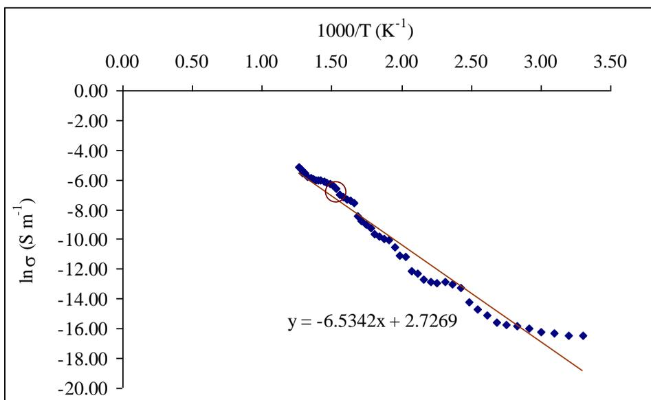
**Figure 10:** (b) Arrhenius plot of the dc electrical conductivity of the SrSnO<sub>3</sub>
