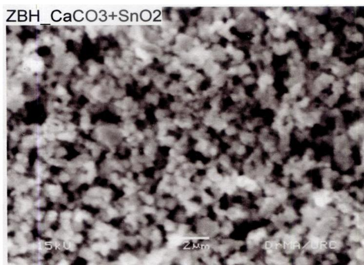
**Figure 7:** SEM micrograph of the  $\text{CaSnO}_3$
