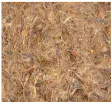
**Figure 3.** Extracted areca nut fiber
