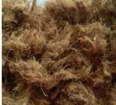
**Figure 4.** Alkali treated areca nut fiber
