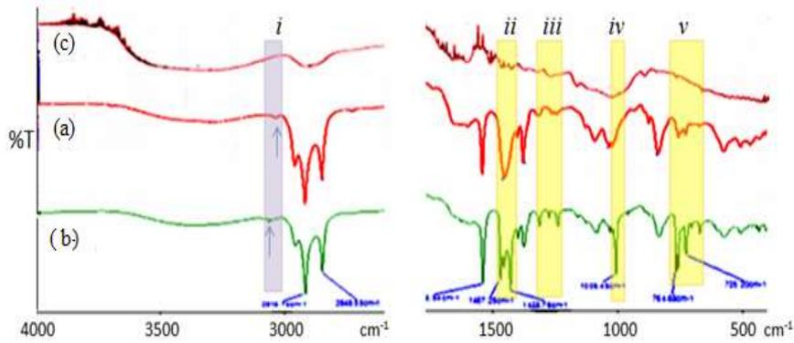
**Figure 8.** FT IR spectra showing (a) rubber (b) alkali treated areca nut fiber-rubber composite, and (c) alkali-treated areca nut fiber
