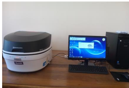
Figure 1 Energy Dispersive X-rays Fluorescence (EDXRF) spectrometer (EDX-7000)
