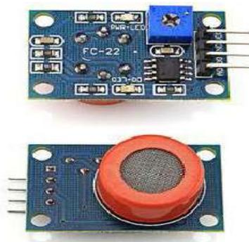
**Figure 4** The photograph of MQ3 gas sensor
