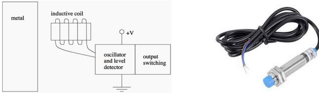
Figure 5 The photograph of inductive detector
