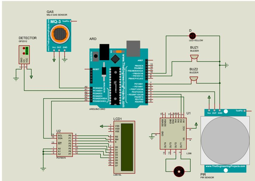
Figure 6 The circuit diagram of Microcontroller Based Automatic Door Opening and Liquid Petroleum Gas detecting system
