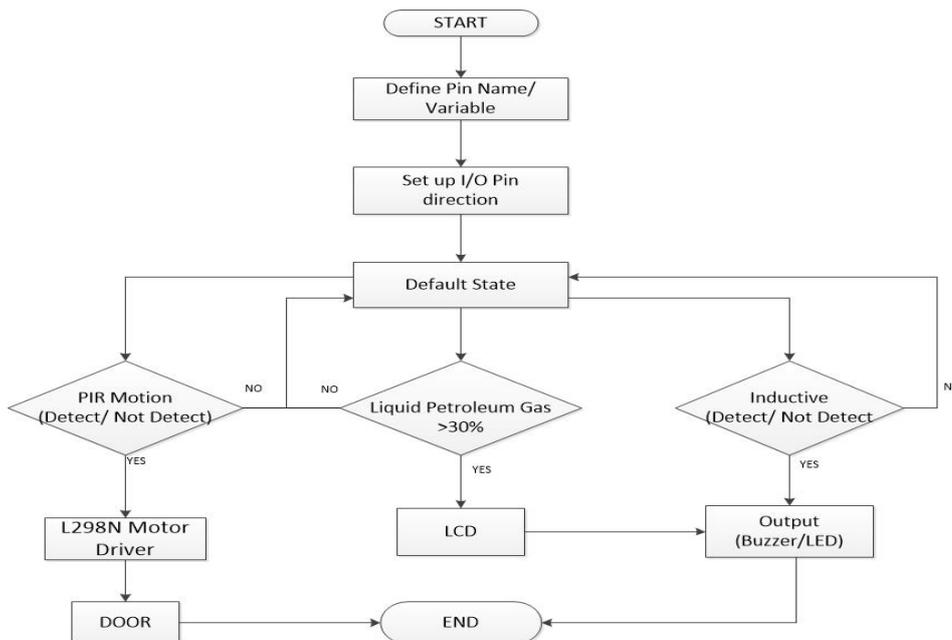
Figure 7 The flow diagram of microcontroller based automatic door opening and liquid petroleum gas detecting system
