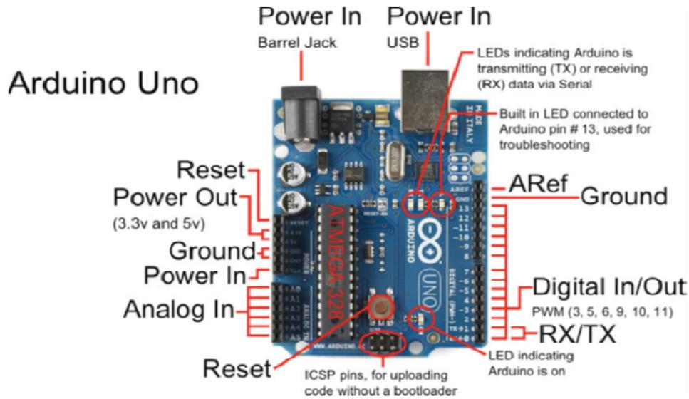
**Figure 2** The pin configurations of arduino uno board
