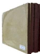
Figure 3 Finished particleboards during conditioning at ambient temperature
